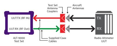
All items required to test radio altimeter systems are included in the ALT-9000 kit.
